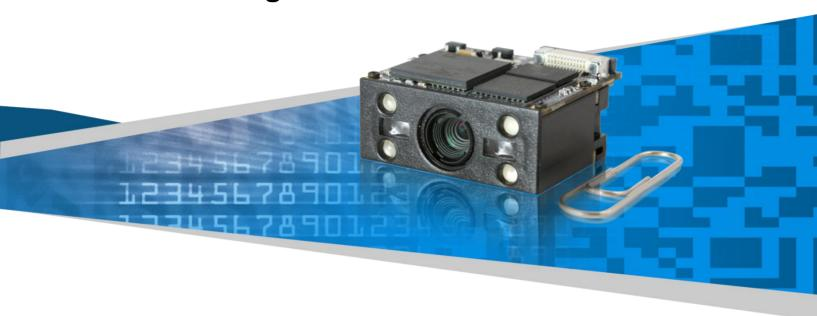
The NLS-EM3000 OEM scan engine, powered by advanced imaging technology and Newland patented **UIMG** technology, a computerized image recognition system, can read barcodes on various mediums such as paper and plastic, with excellent motion tolerance.
