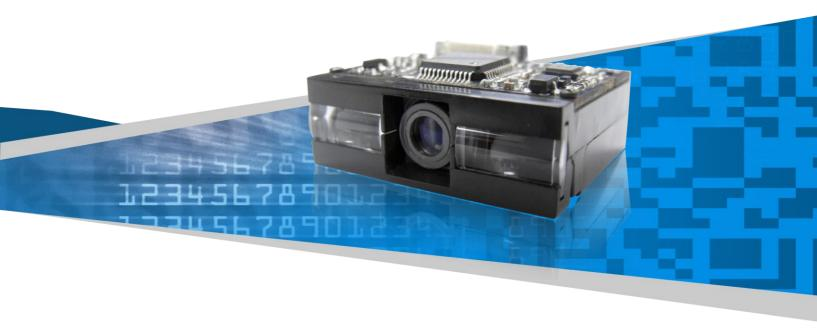
Designed for OEM applications, this high performance scan engine can easily be integrated into various solutions such as kiosks, ticketing machines, PDAs and many more.
